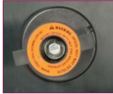
Wire spool hub with locking assembly
