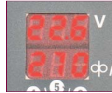
Digital display meter, wire feed speed (IPM or MPM), amperage, voltage, arc time and memory hold
