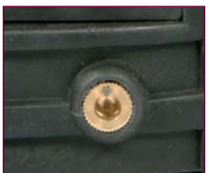
Voltage sensing connector, 25mm dinse
