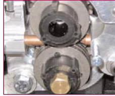
Quick change drive rolls, no tools required
