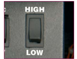
High/low wire feed speed switch
