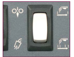
Inch and Gas purge switch
